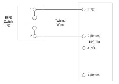
**NOTE** REPO switch rating is 24 Vdc, 1A minimum.
